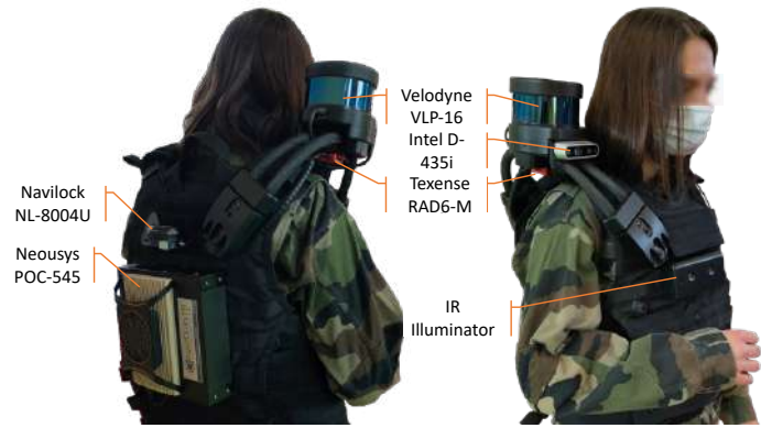
Fig. 2. Tactical waistcoat hardware configuration.
